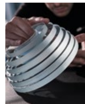
Gluing of the glass sheets.
